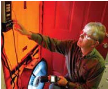
The Minneapolis Blower Door™ airtightness testing system.
