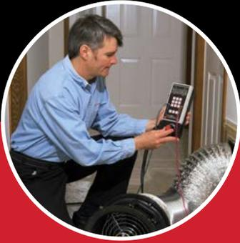
The **Minneapolis Duct Blaster®** is used to measure the airtightness of ductwork.
